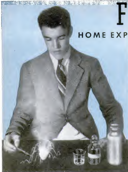
A drop of water acts as a catalyst to produce this spectacular reaction between iodine crystals and metallic aluminum powder
